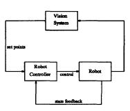
Figure 1: Dual-loop visual servo
