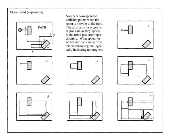
partitions corresponding to the x-position sensor and the move-right action for the first 200 time steps of the experiment. The outermost rectangle shown depicts the sensor extremes as known to the robot. The actual regions extend into infinity at the edges of this rectangle.
