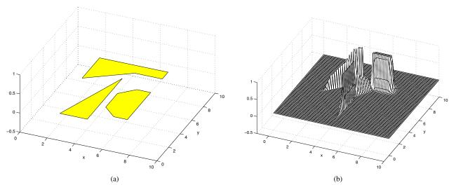
Fig. 1. Validation of the biasing scheme: experimental obstacle layout in (a) and the corresponding passage potential function in (b).
