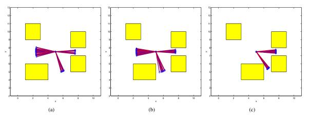
Fig. 2. Experimental validation of the biasing scheme: images showing different obstacle settings together with the robot at all the biased sampled configurations (no unbiased samples in these simulations). The behavior of the biasing scheme is as expected.
