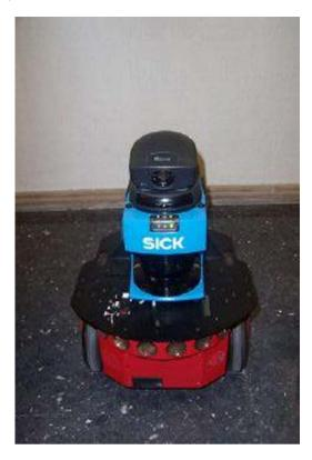
Fig. 10. Indoor mobile robot and sensors.
