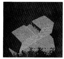
Fig. 13. Composite light-stripe image from the first experiment.
