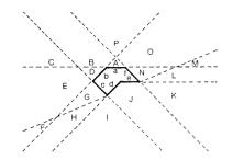
Fig. 7. Regions which view the different aspects of the rightmost object of Fig. 1.
