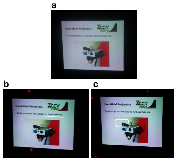
Fig. 5. Light stylus application showing underlining and drawing a box on a slide presentation.
