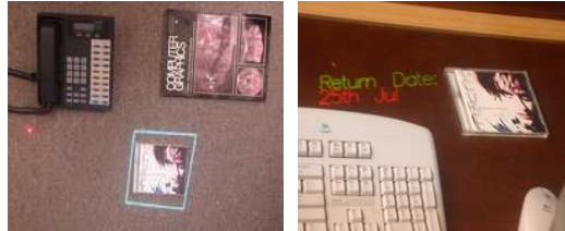
Fig. 6. Electronic sticky note - (a) object selection for attaching a note, (b) retrieval of note.
